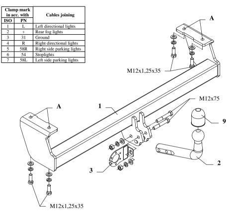
This towbar is designed to assembly in following cars: **SUZUKI GRAND VITARA, 3/5 door,** produced since 09.1998 till 2005 and **SUZUKI GRAND VITARA XL-7** produced since 2001 till 2006, catalogue no. **W08** and is prepared to tow trailers max total weight **1850 kg** and max vertical load **80 kg**.
