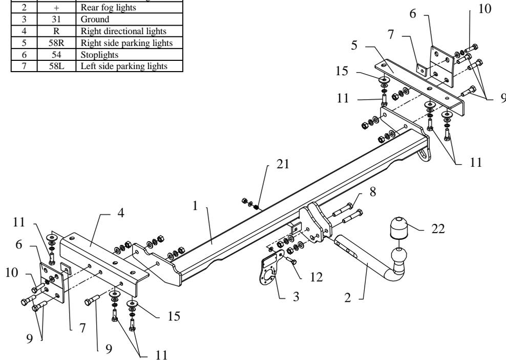
This towbar is designed to assembly in following cars: **TOYOTA LEXUS RX300** produced since 2000 till 2002, catalogue number **O62** and is prepared to tow trailers max total weight **2200 kg** and max vertical load **75 kg**.
