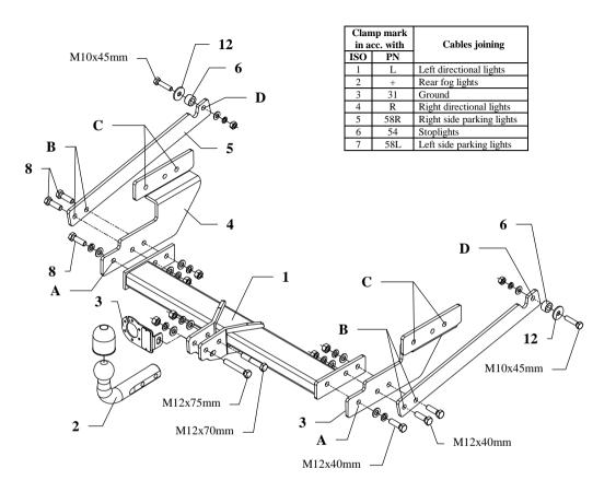
This towing hitch is designed to assembly in following cars: **VOLKSWAGEN T4 - TRANSPORTER**, produced since 1996 till 12.2002, catalogue no. **K27** and is prepared to tow trailers max total weight **2500 kg** and max vertical load **100 kg**.
