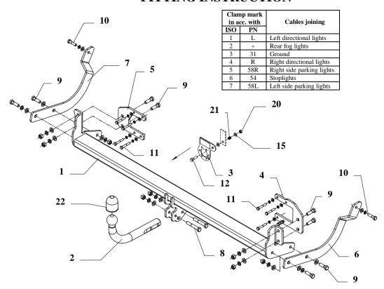
This towbar is designed to assembly in following car: **PEUGEOT 407SW (ESTATE),** produced since 2004 till 08.2008 (**Attention! Not suitable for car with 3.0 HDi V6 engine!**), catalogue number **F28** and is prepared to tow trailers max total weight **1900 kg** and max vertical load **65 kg**.
